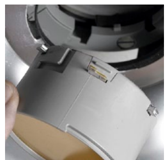
LED module includes ballast and can easily be changed using the bayonet mount.
